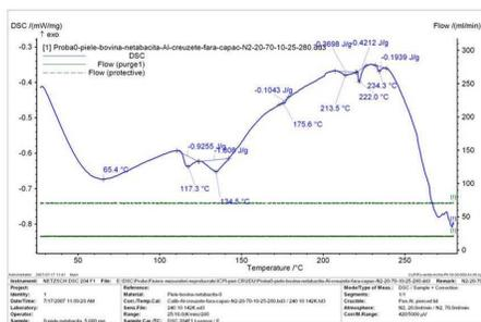
**Figure 6.** DSC curve (obtained in nitrogen flow) hides titanium tanning
