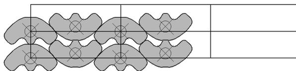
**Figure 6:** Nesting general aspect, obtained by repeating the elementary cell
