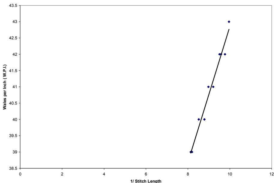
**Figure 2:** 1/Stitch Length (1/l) vs. Wales per Inch (W.P.I.) with trend line
