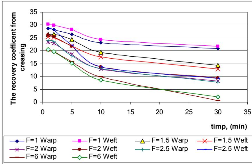
Figure.2. Variation of recovery coefficient from creasing for the studied wovens
