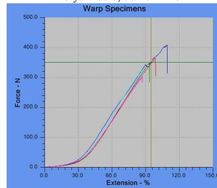
**Figure 8:** Bamboo+Viscose, 34/1 Nm + Polyamide 6, 78/20x2 Den
