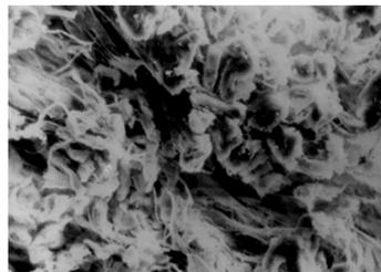
**Figure 9.** Electron microscopy (SEM) photos for bovine leather tanned with the Ti - Al
