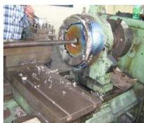
b) Cutting and shaping the ingots
