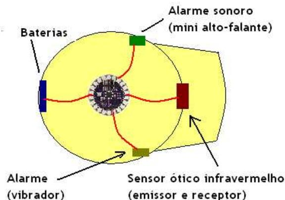
Figure 1: Scheme of the sensor cap.
