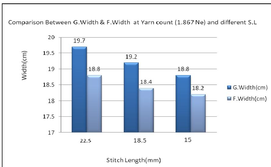
**Figure 2:** Stitch length Vs Width at yarn count, 1.867 Ne
