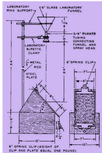
Figure 3: Impact penetration tester
