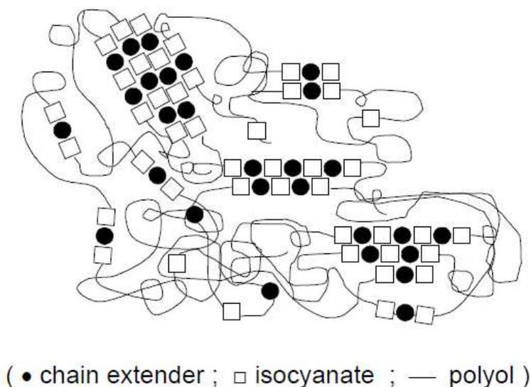
**Figure 1:** Micro-structure of a polyurethane block copolymer
