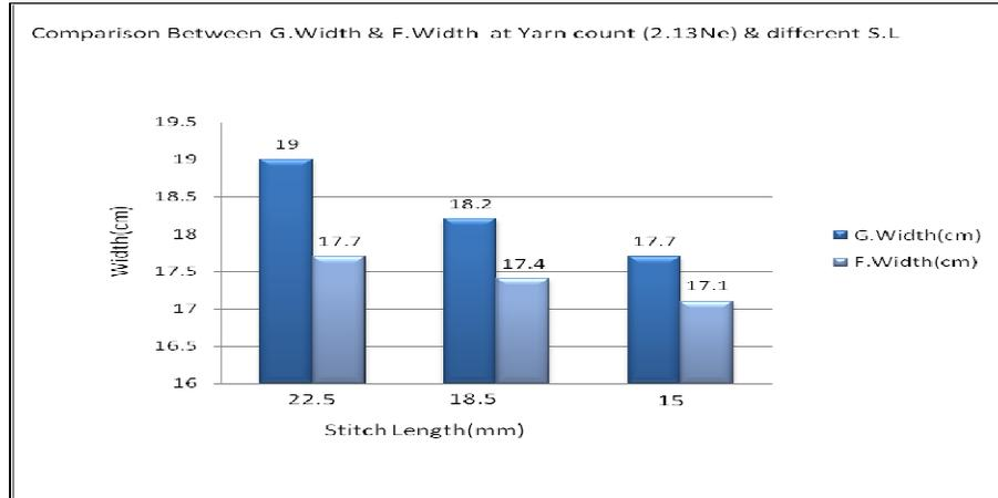
**Figure 3: Stitch length Vs Width at yarn count, 2.13 Ne**
