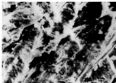
**Figure 8.** Electron microscopy (SEM) photos for pickled (untanned) bovine leather
