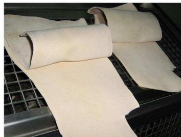
**Figure 5.** Leather tanned with the new tanning materials subsequently split
