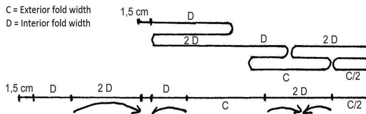
Figure 3b. The distribution of folds at the back
