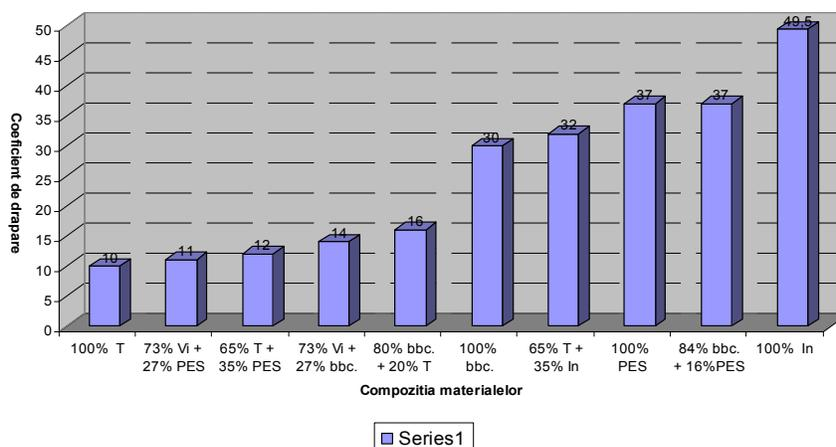
**Figure 3 – Cloth covering coefficient (%) of the analyzed materials**
