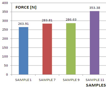
**Figure 13:** Strength graph for samples 1,7,9,11
