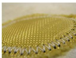
Figure 3: Gold coated para-aramid textile electrode pads
