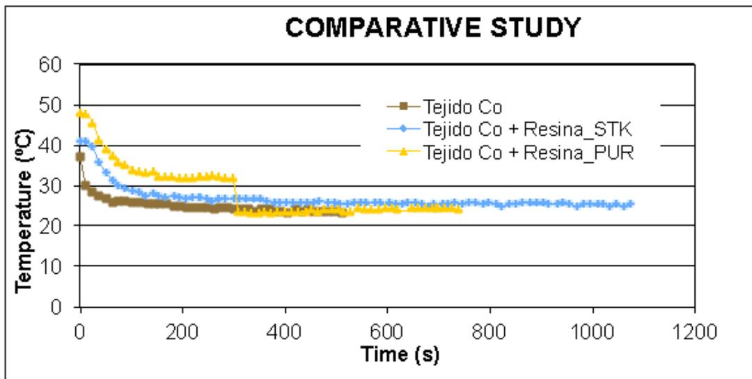
Figure 3. Thermal behaviour of fabrics.
