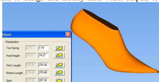
**Figure 4.** The dimensions of the shoe last with the option to reshape a last
