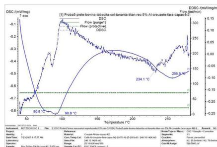
**Figure 7.** DSC curve for the leather tanned with the solutions containing
