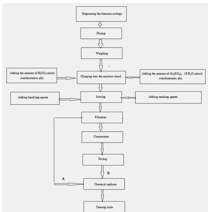
**Figure 2.** Chemical synthesis pathway for obtaining the new tanning agents based on Ti and Al
