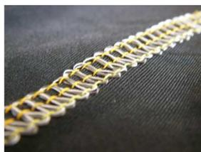
Figure 2: Elastic stitch of conductive threads
