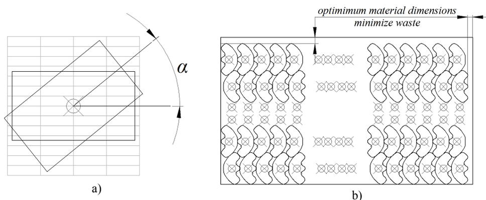
**Figure 7:** Testing different material positions over the row of elementary cells *a*, in order to retain the position with the highest material usage factor *b*
