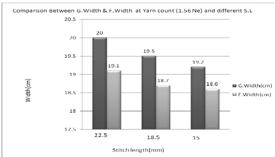
**Figure 1:** Stitch length Vs Width at yarn count, 1.56 Ne
