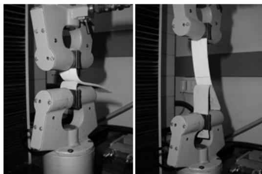
**Figure 4:** Example of quality control tests (adhesion)
