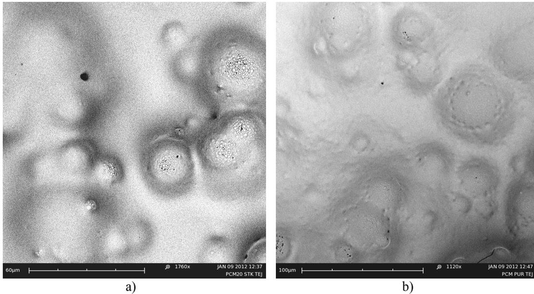
Figure 2. PCM on cotton fabric surface after coating.
