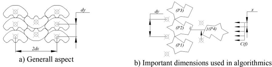
Figure 3: Variant 2 used to generate nesting layouts
