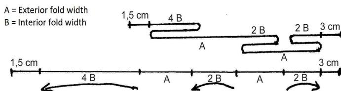
Figure 3a. The distribution of folds at the front
