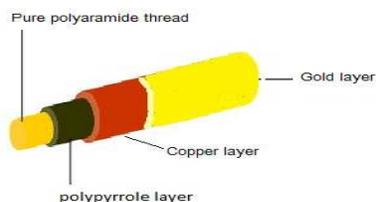
Figure 1: Schematic presentation of coated thread.
